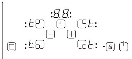
As the temperature drops, the 't' displays will be erased and the hob control unit falls back into the S mode. This means that the user can reactivate the appliance by touching
