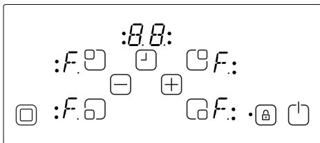
The safety turn-off causes the hob control to be turned off and to switch to the S mode. An 'F' will flash in all heater displays.
